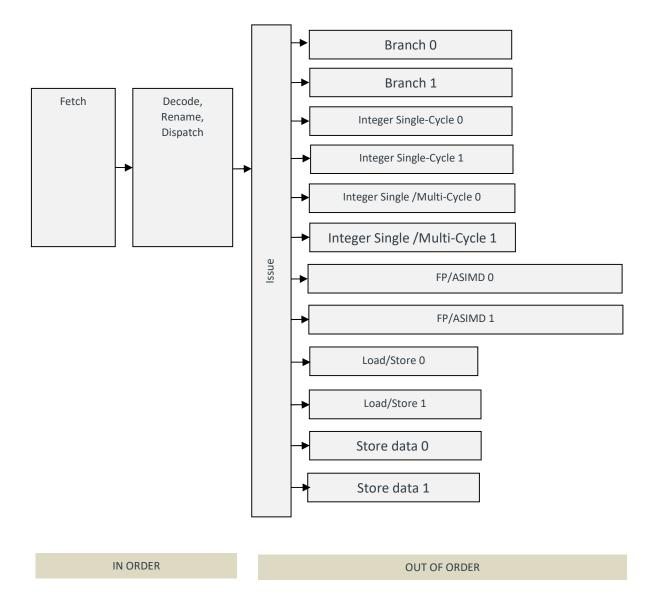
The execution pipelines support different types of operations, as shown in the following table.
